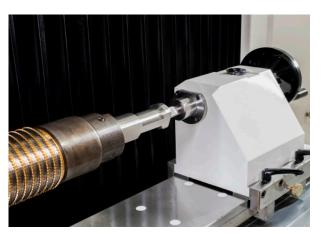
Standard screw actuated tailstock allows for the precise work between centers. Rail mounted, the tailstock can be easily moved to accommodate different setup lengths.
