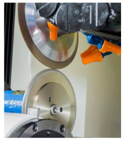
The wheel truing cycle is programmed into the machine. Simply enter the amount of stock removal and the machine automates the cycle.
