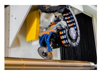
6-Axis design allows for (3) rotary motions and (3) linear motions and are simultaneously controlled allowing for the manufacturing and re-sharpening to today's most demanding designs.
