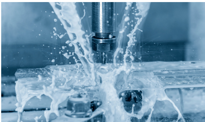
Flood Coolant System
